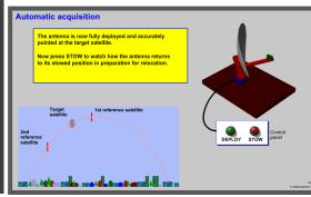
Auto-deploy and stabilized antennas are explained using 3-D animations, giving operators of these mobile terminals the understanding for troubleshooting. SUMMARY: Fundamental theory of VSAT communications for all VSAT technicians and engineers.
